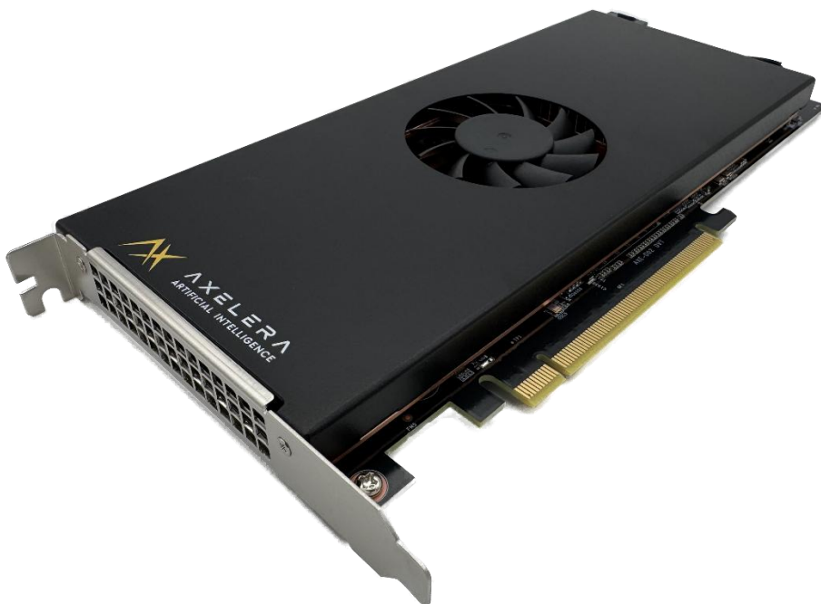
Figure 1: Axelera AI Metis PCIe 4-AIPUs AI Accelerator Card with active cooling
