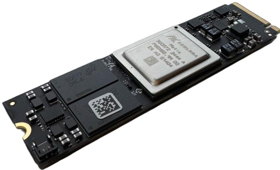
Figure 1: Axelera AI Metis M.2 Max card AI module fits to systems with an NGFF socket
