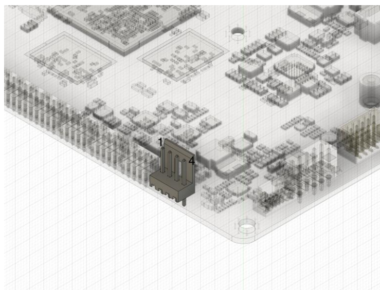
Figure 12: Detail of Metis Compute Board showing pin numbering for ON/OFF and RESET buttons
