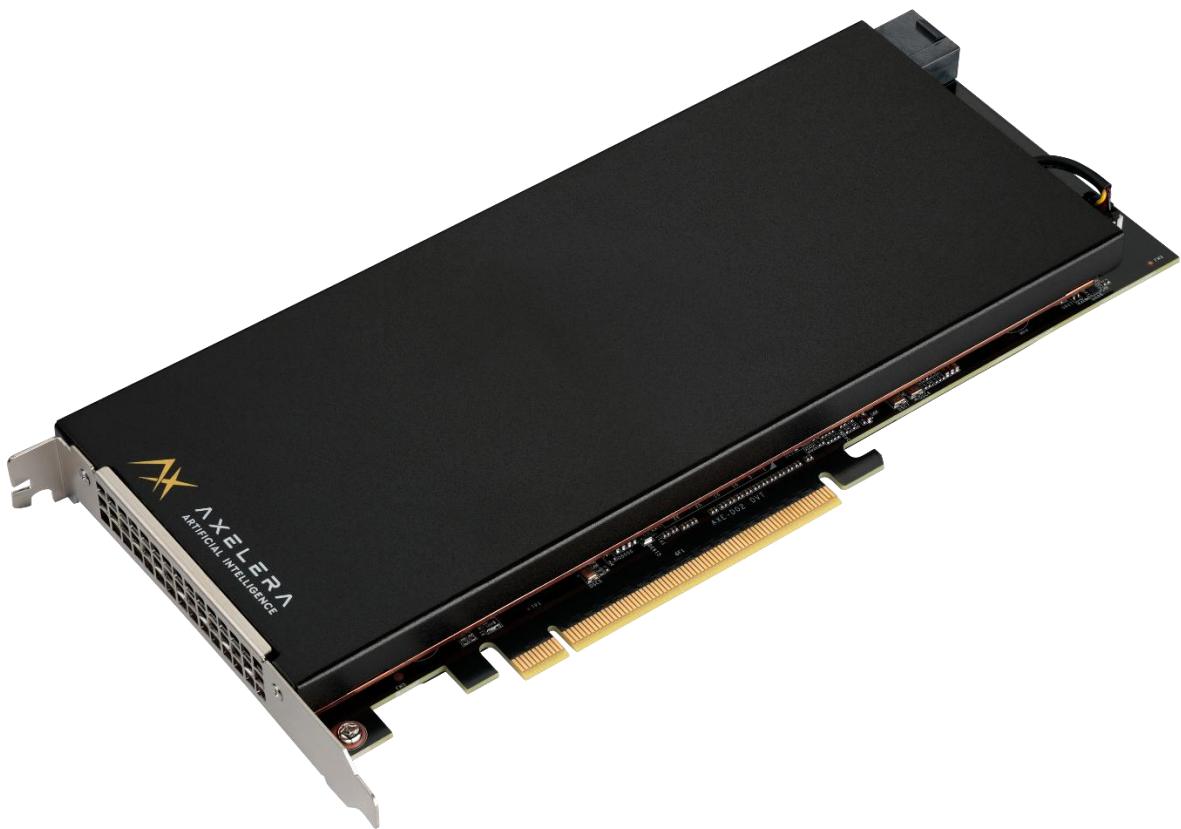
Figure 2: Axelera Server 150p with passive cooling
