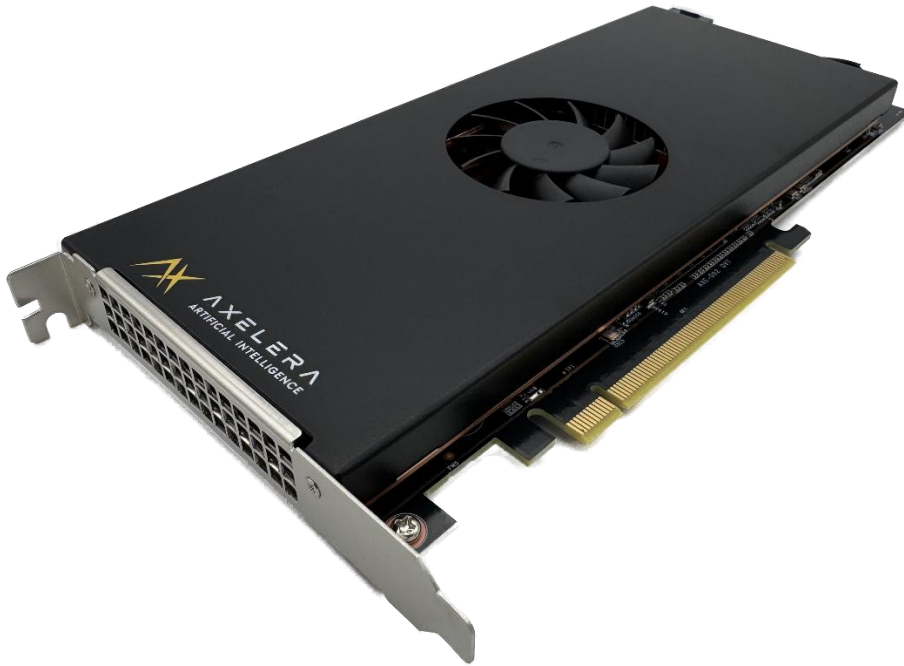
Figure 1: Axelera Server 150p with active cooling
