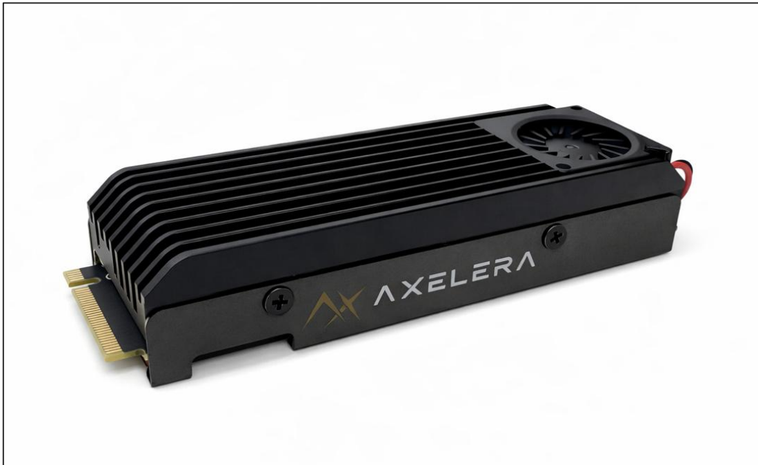
Figure 4: Axelera Embedded 113m active cooling solution (heatsink with blower fan forced air)
