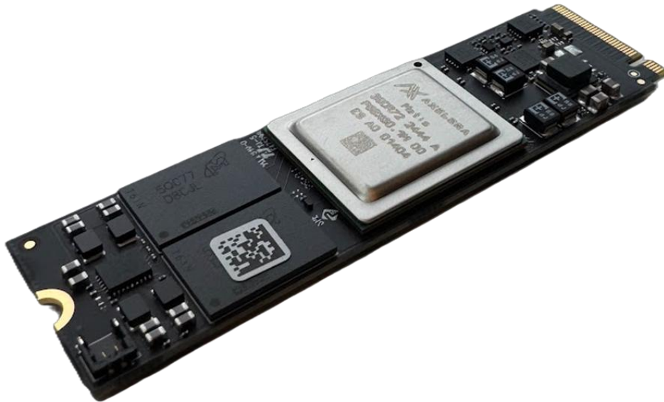
Figure 1: Axelera Embedded 113m card AI module fits to systems with an NGFF socket
